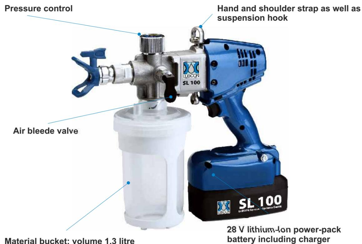
The 75 cm long nozzle extension allows an ergonomic adjustment of the device to any body size. Thus, the lubricator **LUBCON SL 100** is an ideal tool for the maintenance of rail route networks.
