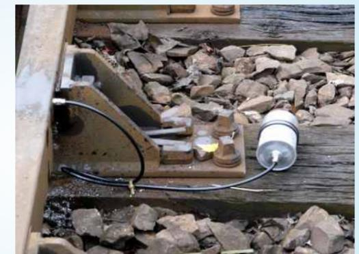
MicroMax® 120 installed at check rail
