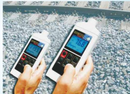
Evidently effective against squeaking and screeching: measurement prior to lubrication (left) and after application of Sintono® Terra HLK (right).
